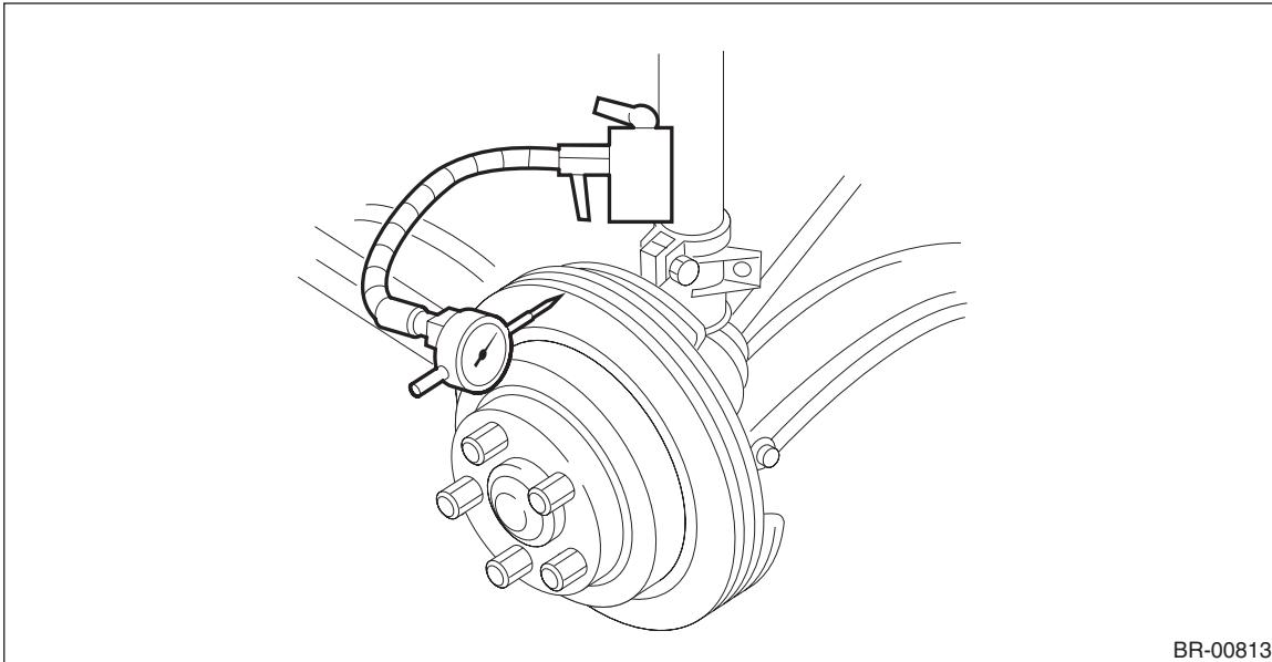
4) If the disc rotor runout exceeds the limit, resurface the disc rotor.
